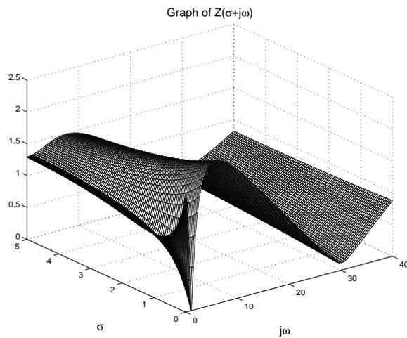
Figure 2:  $Z(s)$  plot for right half plane
